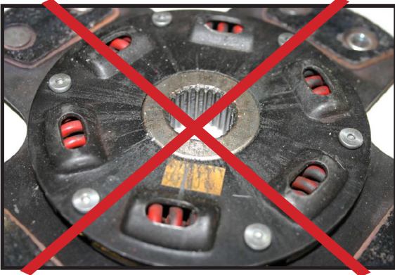
Example of TOO MUCH GREASE, which causes grease to spray all over the disc and ruin the disc material or pads.
