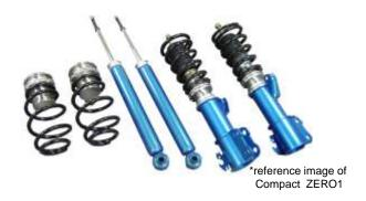
♦ Well requested Negative camber spec for Compact series now will be released. To install this, Front camber is attached on fitting hole of knuckle bracket. Byhaving negative camber spec suspension, front grip is improved during cornering, which can improve time on track/circuit driving.
