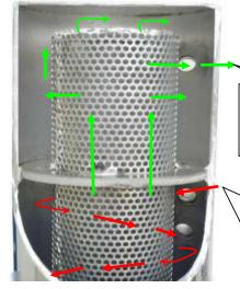
The gas which go through filter is purified to reduce the amount of foreign matter.
