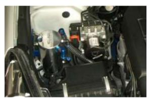
♦ This catch tank manage blow-by-gas which return to intake, so engine will receive fresh mixing air which is less foreign matter. It prevents reblow of blow-by-gas which prevent going engine power down.
