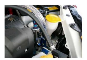
♦ This catch tank manage blow-by-gas which return to intake, so engine will receive fresh mixing air which is less foreign matter. It prevents re-blow of blow-by-gas which prevent going engine power down.
