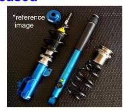
♦ It's designed based on ZERO1 which offers sporty taste driving feel while keep comfortable ride feel. This is added 8 steps rear damping force adjustment kit which is enable to adjust ride feel depend on number of passenger or luggage.
